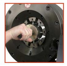
The die size stamped on the face of the die should face toward the operator
