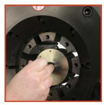
Bring the crimper head to a fully closed position and remove the die insertion tool.
