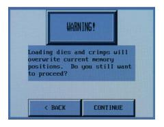
Some hose and fitting manufacturers furnish a complete set of crimp specifications which can be downloaded into the crimper memory. Prior to downloading, a warning screen will appear warning that all previously entered settings will be lost.
