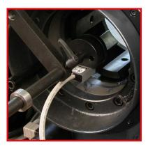
An electronic Coupling Stop is available. Set up is identical, but when the fitting touches the Coupling Stop, the crimp cycle will start automatically.
