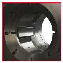
Install Intermediate Adapter Dies as shown previously making certain that the Intermediate Adapter Die I.D. matches the Hydraulic Die O.D.
