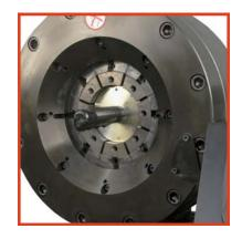
Proceed to the AccuCrimp operating instructions to set up the crimper for the hose and fitting being crimped.
