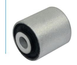
Control arms as well as many other suspension and steering components is fastened to the chassis through bushings. Dayco bushing parts are designed to reduce noise and vibration from the road while providing the necessary connection to the vehicle. The rubber compounds used in their manufacturer ensure long lasting resistance to cracking.
